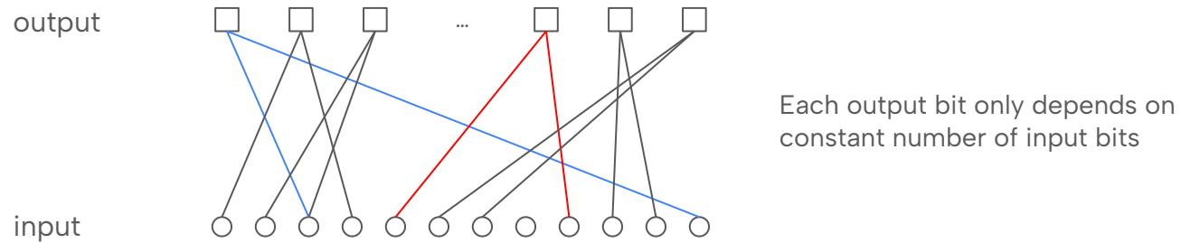
NC0 class: Functions definable by Constant Depth Circuit with bounded fan-in gates
